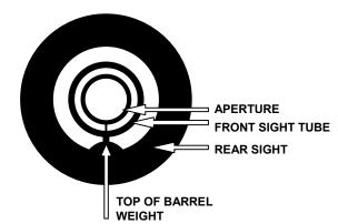
Proper sight alignment is a matter of centering the front sight hood in the rear sight. The hood will not quite fill the rear sight and cadets will be able to see light around the outside of the hood; we call this a "line of white".
