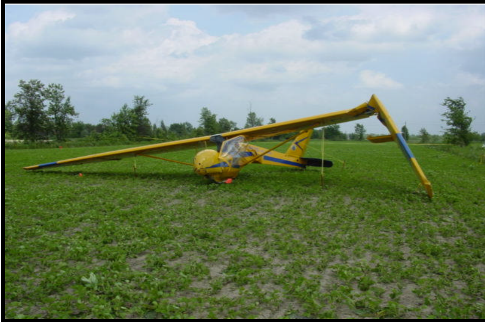
Photo 2: Left Wing Damage
