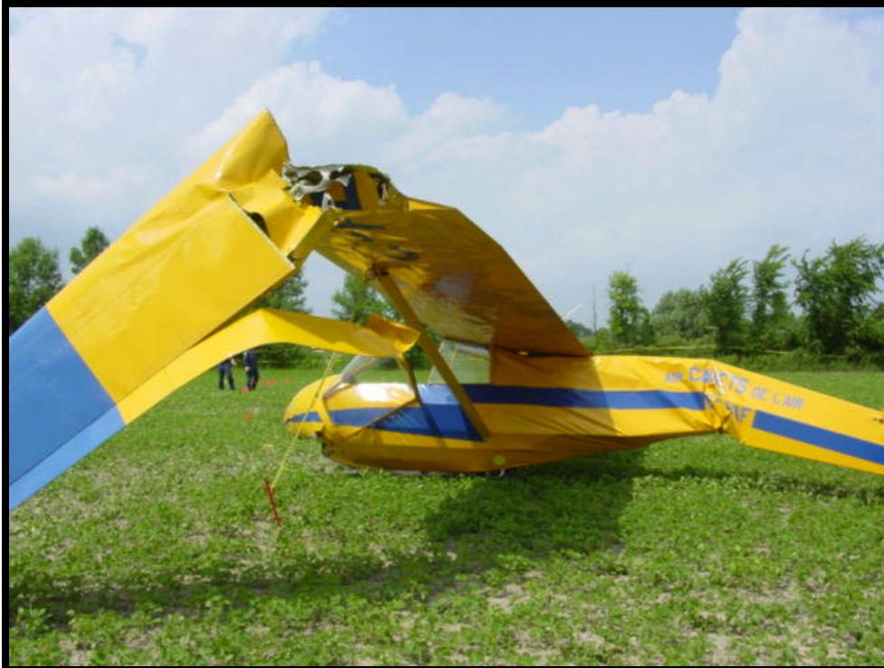
Photo 2: Left Wing Damage
