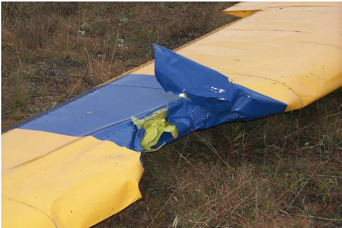
Photo 4 Impact Damage - Right Wing
