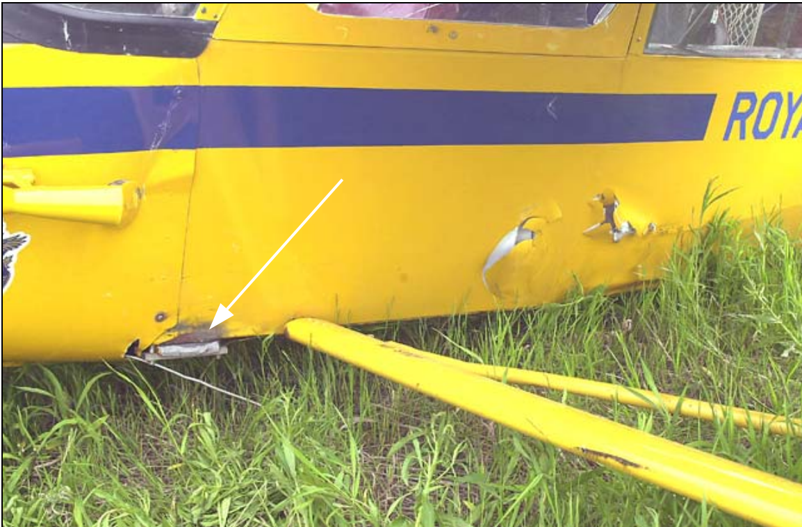
Photo 2: Broken gear leg and fuselage damage
