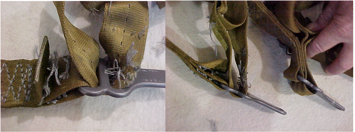
Fig 9, 10. Broken stitching, left lower harness lock; comparison with serviceable lock.
