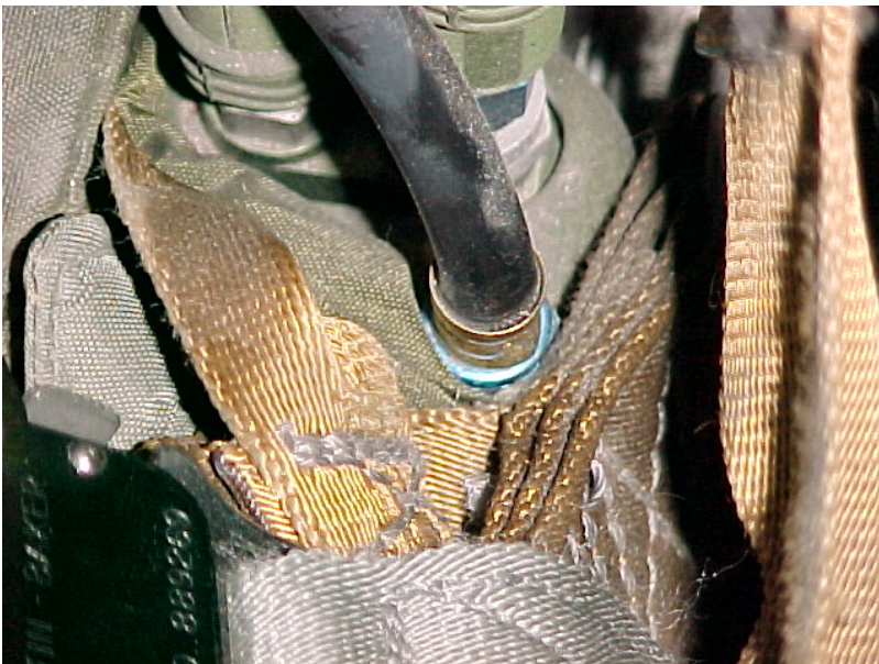
Fig 11. Oxygen attachment pipe nut location vs. lower harness lock stitching.
