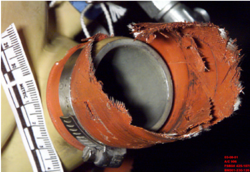
Photo 3: ECS rubber hose located between the ECS turbine and the Anti-ice add heat valve.
