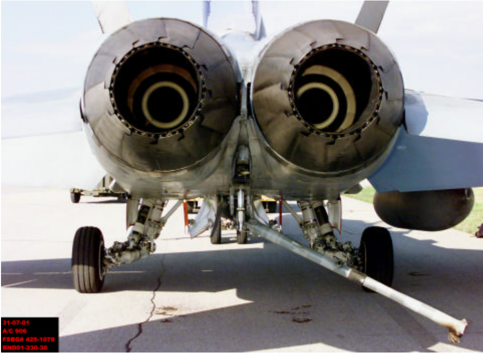
Photo 1: Damage to tail hook and nozzle area.
