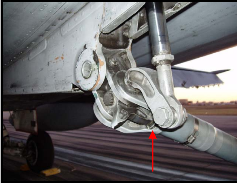
Photo 5: Stop Arrestor Hook Assembly Showing Cracked Gear Bearing Sleeve Assembly
