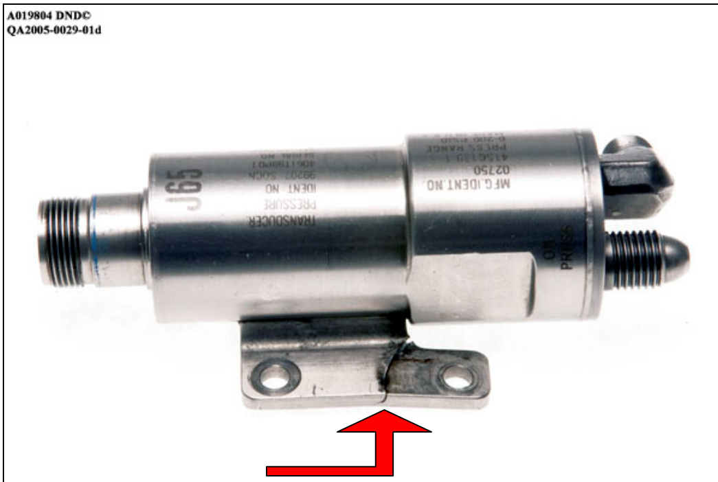
Photo 6: Oil Pressure Transmitter
