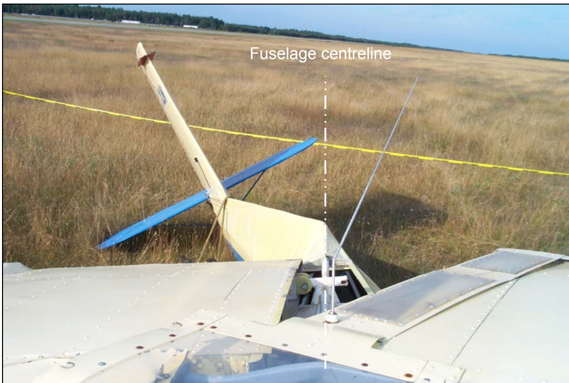
Photo 4: Rear fuselage damage
