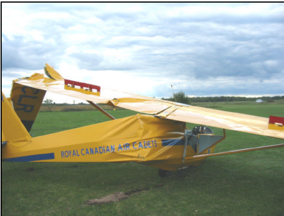
Photo 6: Note that the spoilers are fully extended.
