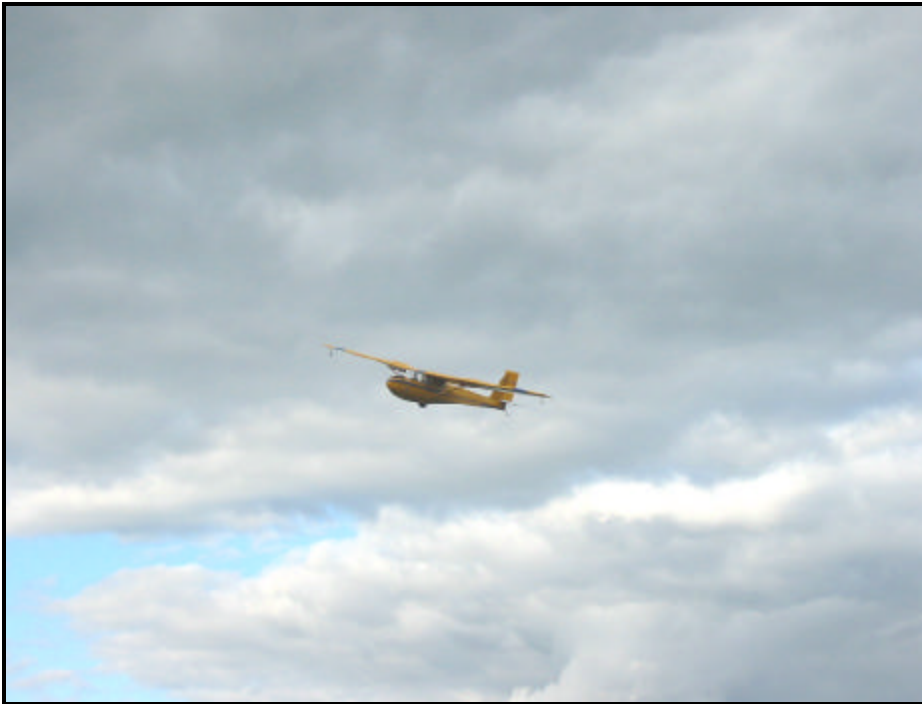
Photo 2: Glider is level at 100' AGL and starting to turn towards the Auxiliary field.
