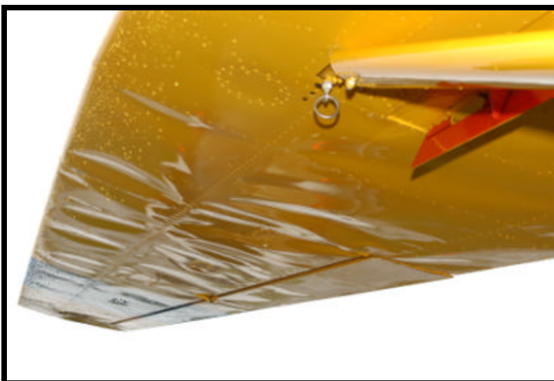
Photo 2: Right Wing Damage
