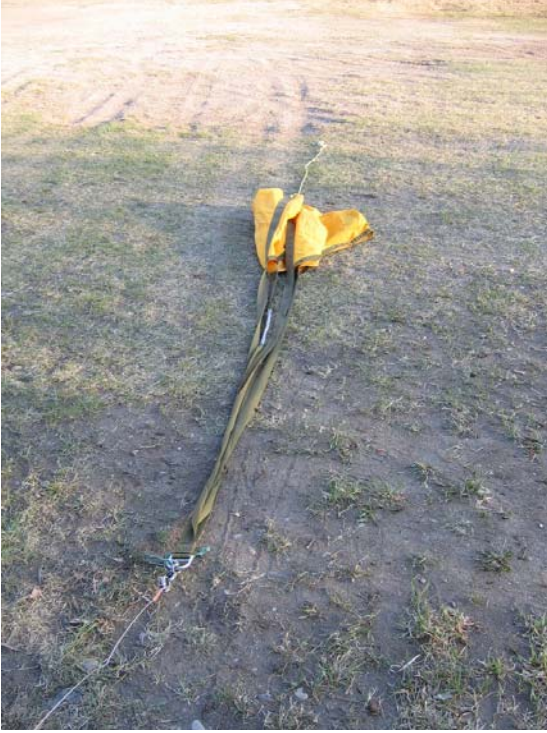
Photograph 3: Cable, Chute, Weak Link
