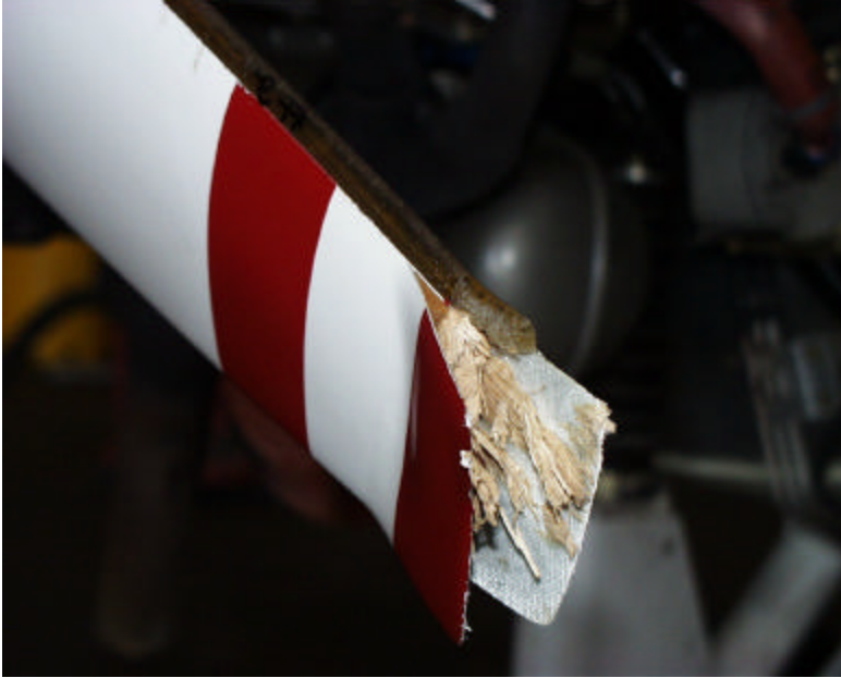
Photo 1: Damage to propeller
