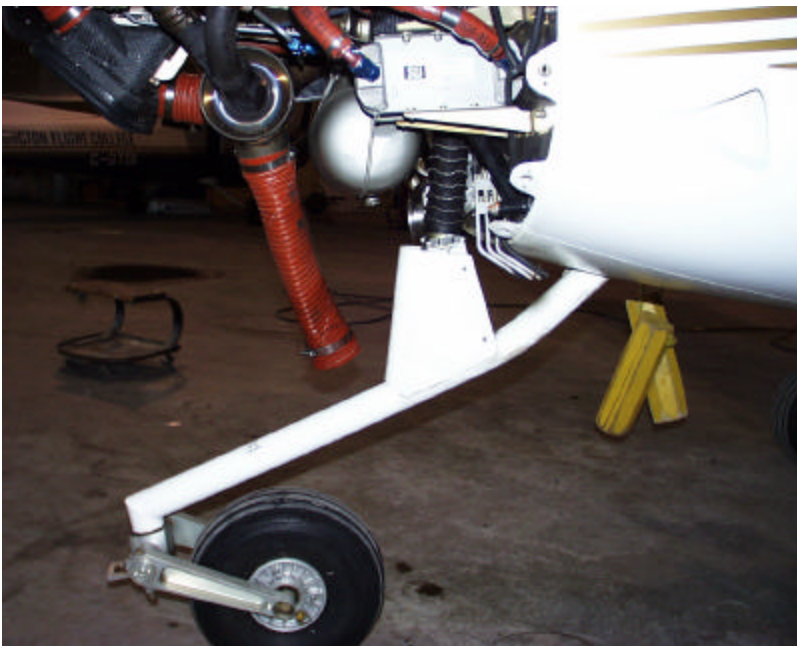
Photo 2: Damage to nose gear shock (overview)
