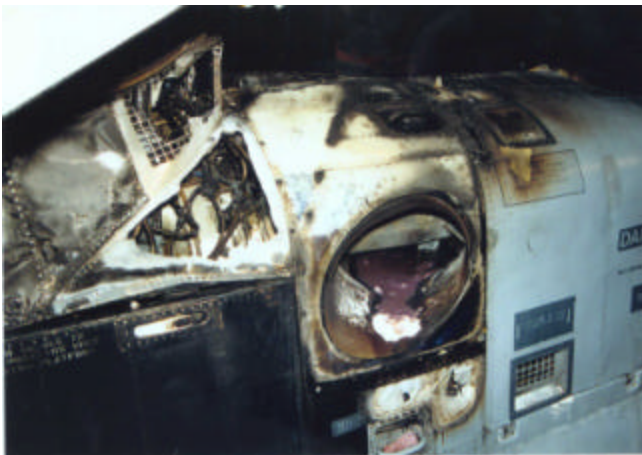
Figure 7 - Fire damage to Engine and Transmission Area
