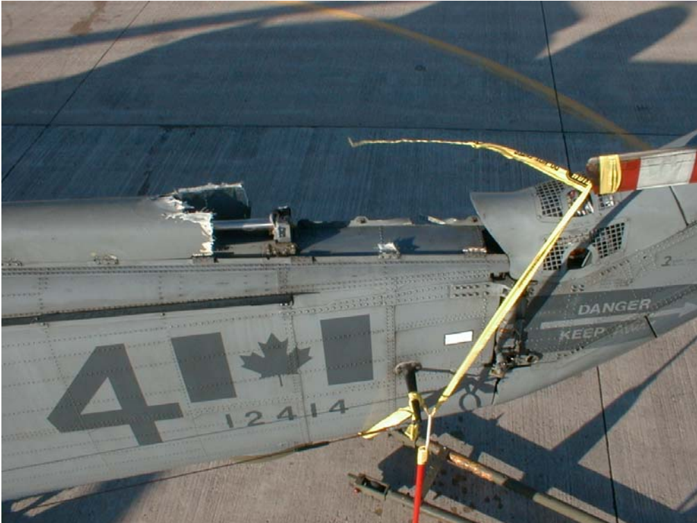
Figure 3 - Tail Rotor Shaft Damage
