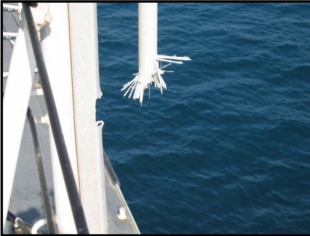
Photo 3: Blade Cut Angle on Stanchion and Antenna
