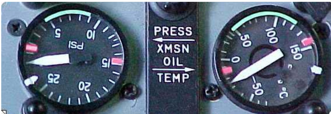
Figure 1- MGB Oil Temperature and Pressure Gauges
