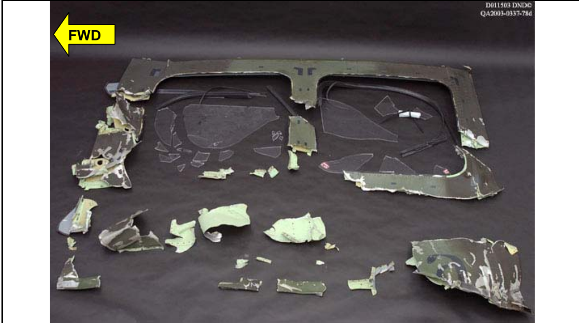
PHOTO 1 Recovered pieces of the LH cargo door of Griffon CH146434.
