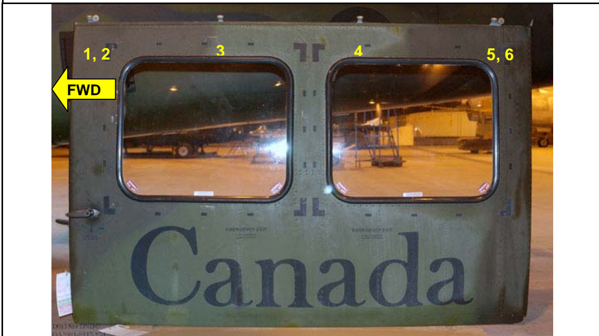
PHOTO 2 Standard CH146 Griffon LH cargo door indicating the roller numbering sequence used.
