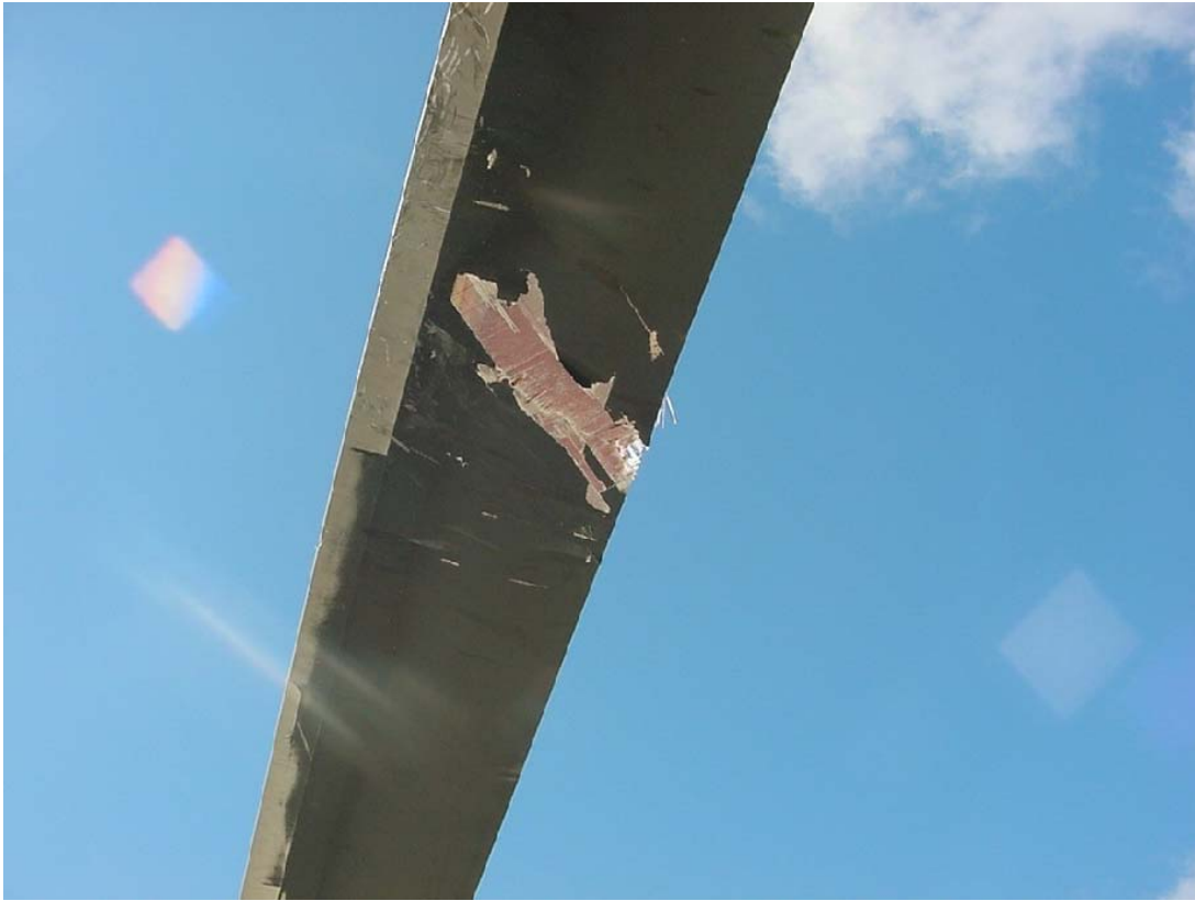
PHOTO 13 Damage to one of the main rotor blade from aircraft CH146434.
