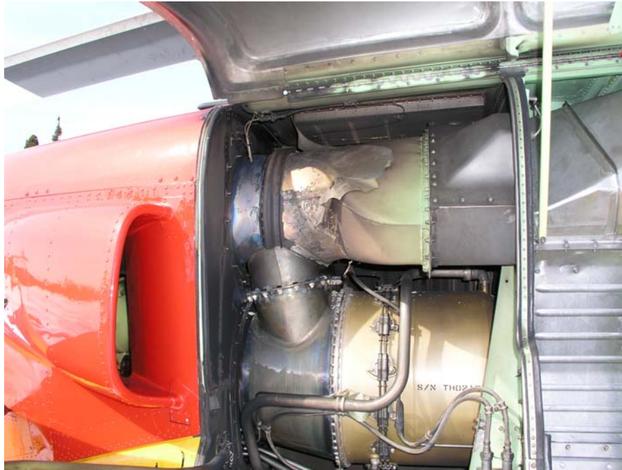
Photo 1: Number two Engine Compartment showing soot, burnt paint and discoloration.
