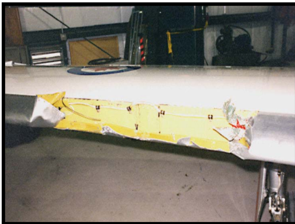
Photo 3 – 114081 closer view of damaged right leading edge
