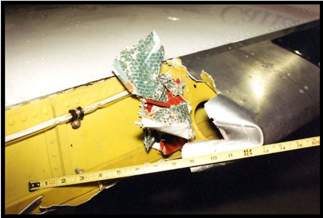
Photo 5 – Portion of 114006 right trailing edge embedded in right leading edge of 114081
