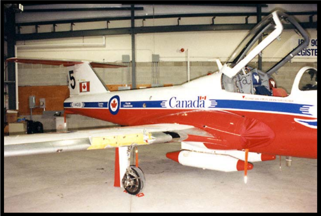
Photo 2 – 114081 showing damaged right leading edge
