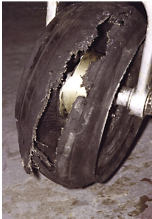
Photo 2: Nose gear and tire damage
