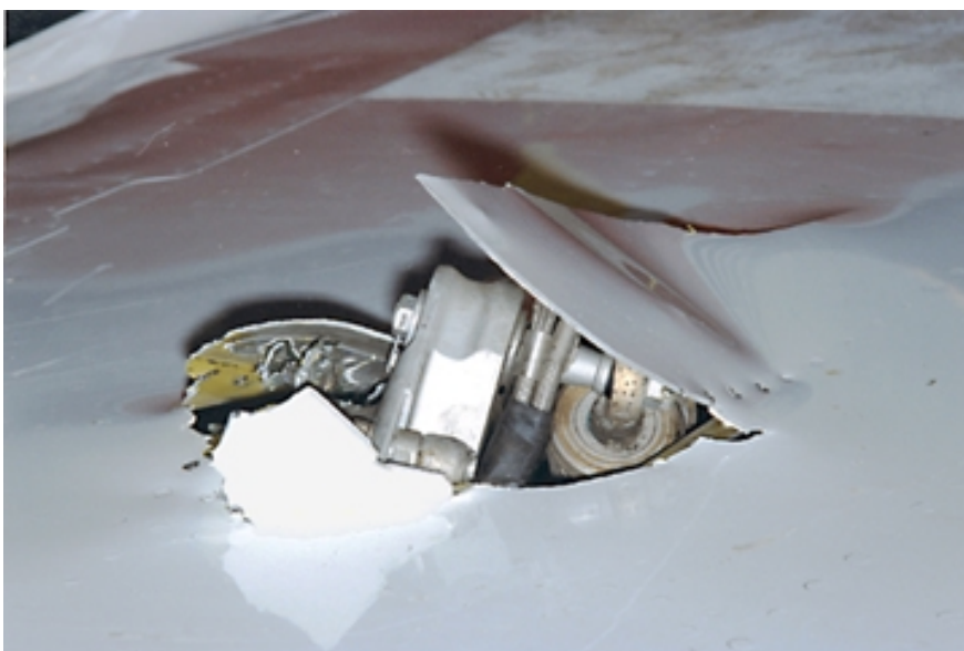
Photo 4: Right –hand main landing gear forced through upper surface of right wing.
