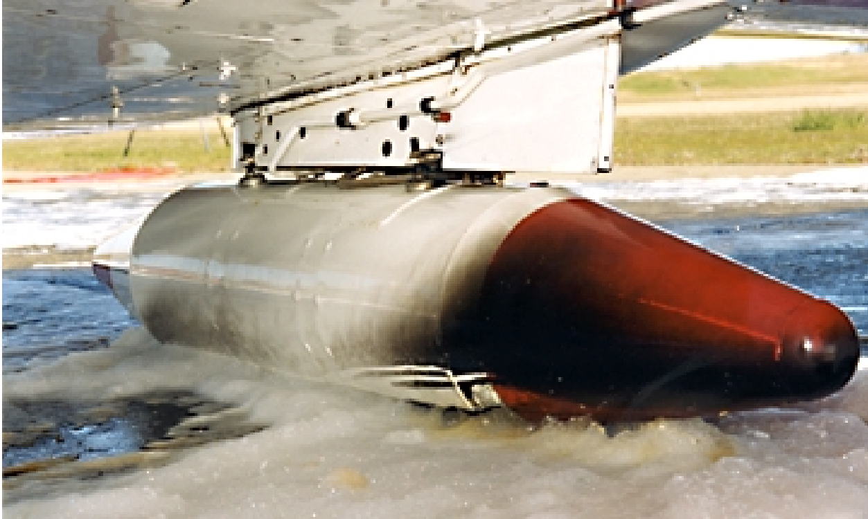
Photo 7: Right-hand smoke tank
