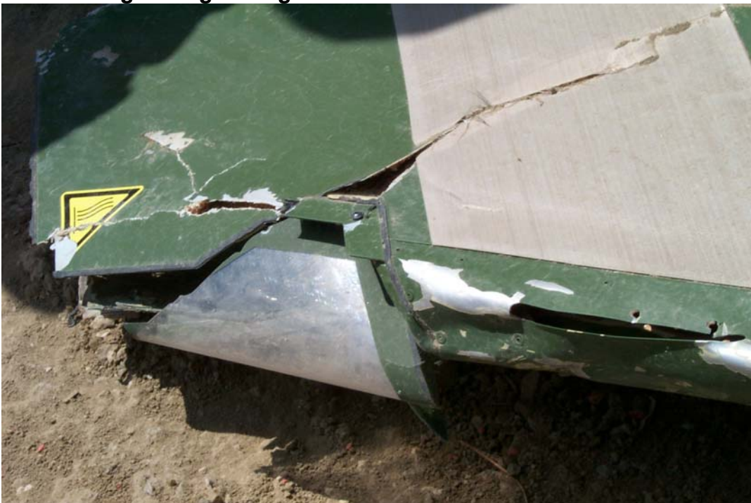
Photo 4: Right wing damage
