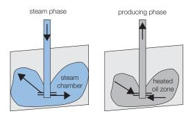
Thermal "Steam-Assisted Gravity Drainage" (SAGD) Process
