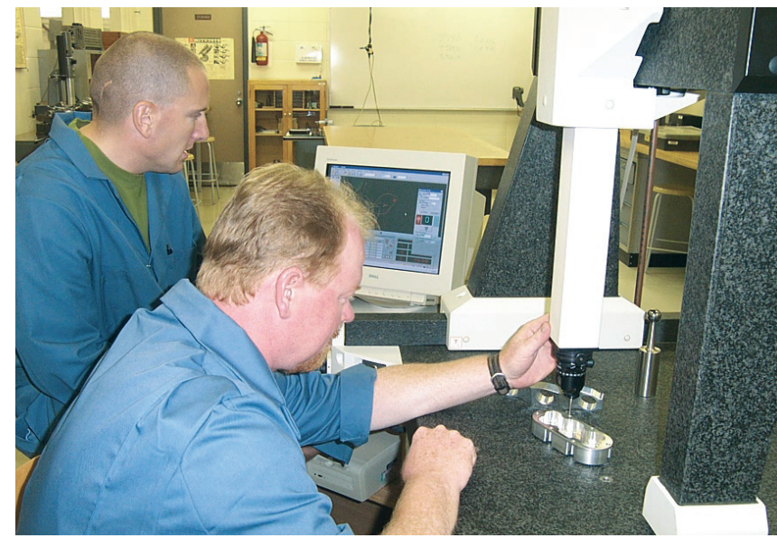
NAIT staff use an advanced metrology instrument that provides measuring accuracy to within millionths of an inch. Such instruments will be available for industry use in the new NAIT Shell Manufacturing Centre.
