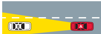
Using the inside rear view mirror – Vehicle A can see Vehicle B
