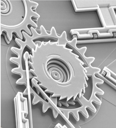
Photograph of a real nanomachine, a ratchet actuator. The device is about 50 microns across - for comparison, a human hair is about 100 microns across.
