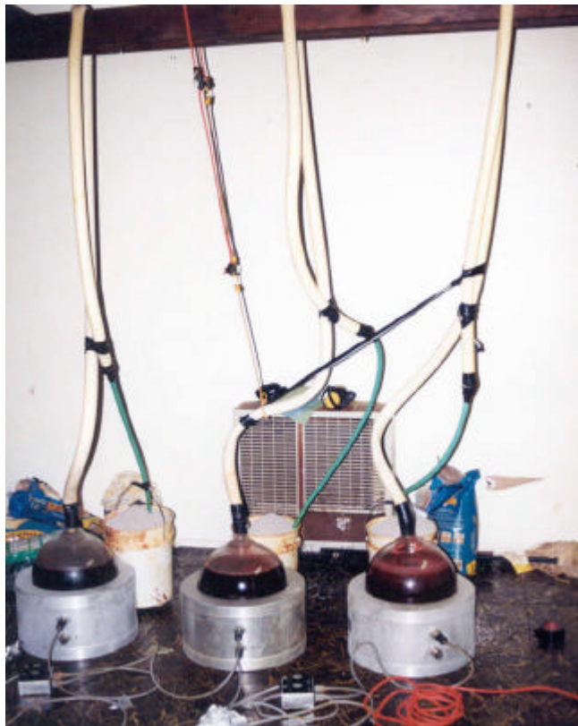
Note the group of round bottom flasks sitting in heating mantles. The vapour exhaust hoses are clearly visible extending from the top of the vessels. Note what appear to be half face cartridge respirators on the top of the heater/air conditioner in the rear of the patio. (Photo 30)
