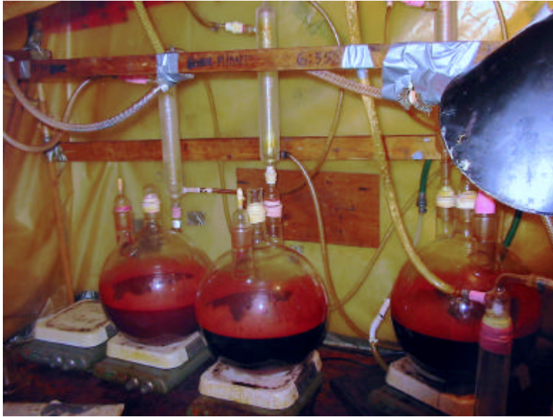
Several large round bottom flasks sitting on heating elements. The red phosphorous solution is clearly visible boiling inside. (Photo 43)
