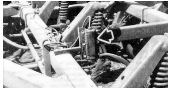
FIGURE 4. Senstek DCM-2 Depth Sensor Mounted on Cultivator Frame.
