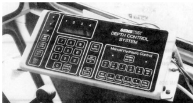
FIGURE 2. Senstek DCM-2 Control Console Mounted in Tractor Cab.
