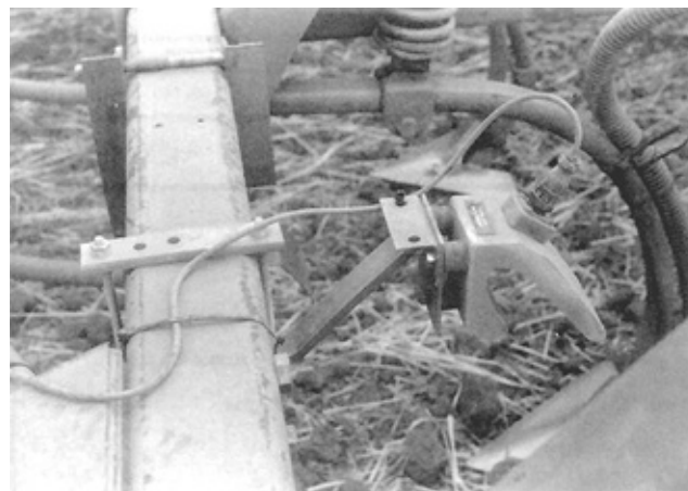
FIGURE 4. Ultrasonic sensor mounted on tillage frame.
