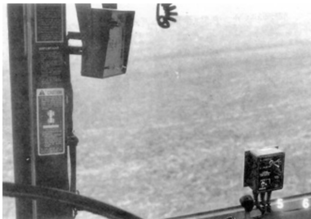
FIGURE 3. Depth control box and controller mounted in tractor cab.
