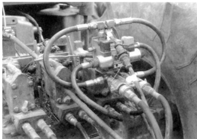
FIGURE 5. Hydraulic solenoid valve mounted at rear of tractor.
