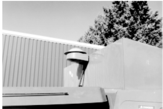
GreenStar antenna positioned on a John Deere 9610 combine.
