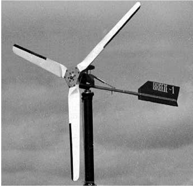
Figure 1. Breeze-1 Aeration Turbine.
