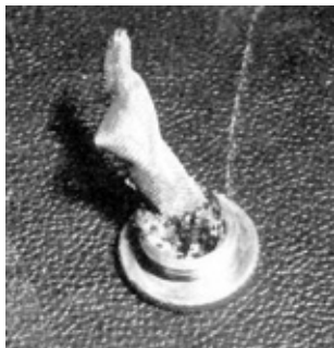
FIGURE 4. Plugged Outlet Nozzle Strainer.
