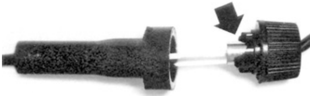
FIGURE 4. Broken Fuse Holder.
