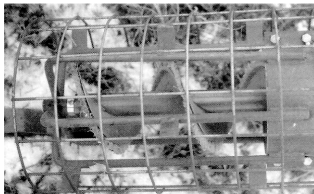
Bristle Flighting Screw Conveyor Inlet: 6 in (150 mm) steel flighting with 1 in (25 mm) nylon bristles on the edge, 8 in (200 mm) conveyor tube, 41 ft (12.5 m) long.
