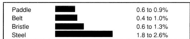
FIGURE 2. Crop Damage, Laird Lentils at 12.8% M.C., One Pass.
