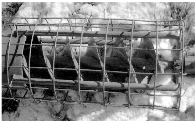
Steel Flighting Screw Conveyor Inlet: screw conveyor with steel flighting, 8 in (200 mm) diameter, 40 ft (12.2 m) long, with double flighting at inlet.
