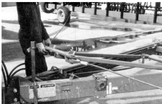
FIGURE 5. Operator Lifting the Wing Cable Pivot Arm for Transport Position.
