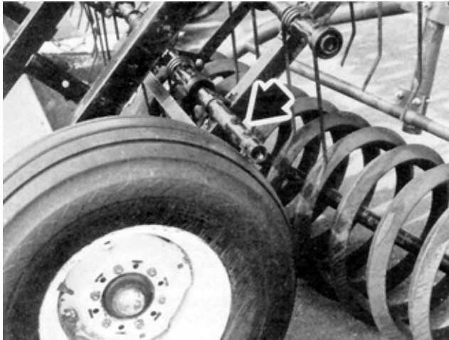
FIGURE 7. Harrow Tine Removed to Prevent Tire Interference with Wing Wheel.
