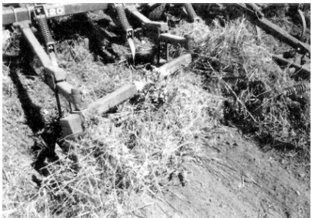
FIGURE 7. Straw Wrapping Around the Weeders When Rotating in the Reversed Direction.
