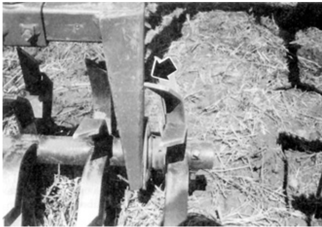
FIGURE 9. Bent Teeth Stopping Rotation.
