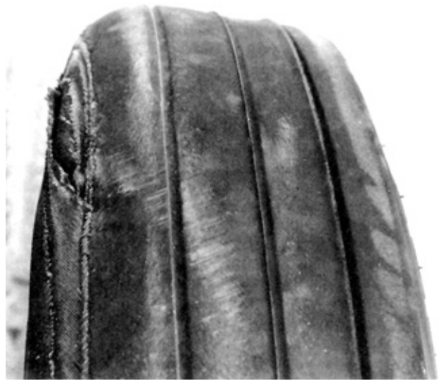
FIGURE 6. Excessive Tire Wear.
