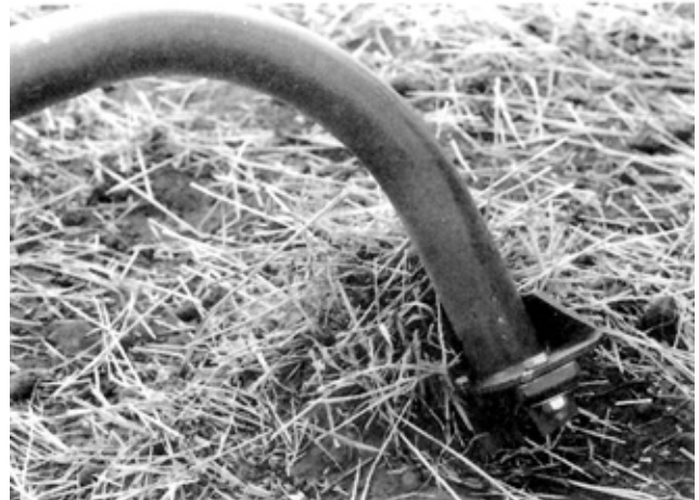
FIGURE 7. Upper: Packer Separation from Packer Draw, Lower: Broken Pillow Block.
