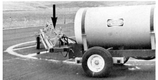
FIGURE 12. Boom Interference when Making Sharp Turns.
