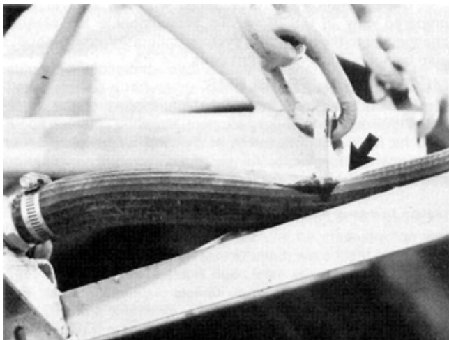
FIGURE 24. Crushed Right Boom Inner Hose.
