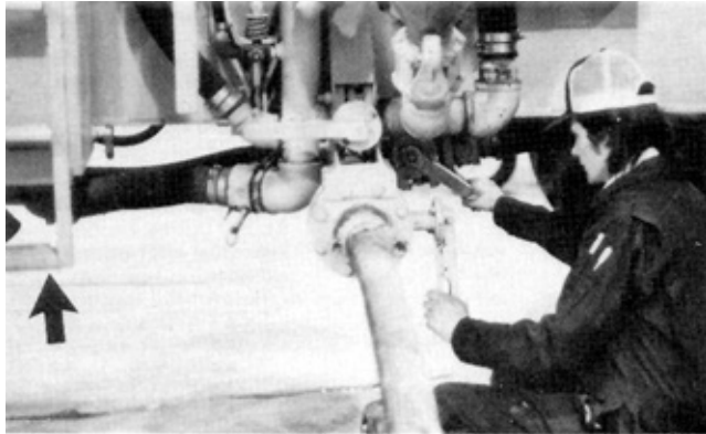
FIGURE 23. Operator Directly Behind Engine Exhaust Outlet when Filling Tank.
