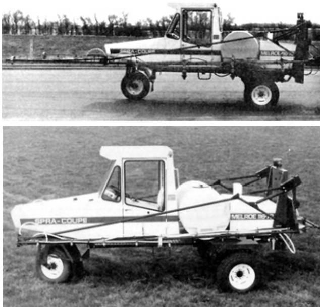
FIGURE 13. Spra-Coupe in Transport Position: (Upper) Partial Transport, (Lower) Complete Transport.
