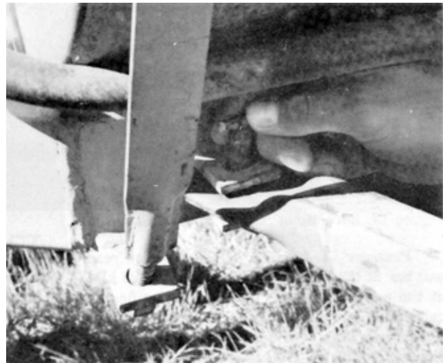
Figure 16. Awkward Location of Radius Brace Pin.
