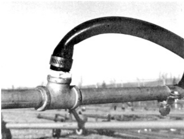
Figure 12. Buckling of Supply Hose at Boom Inlet.
