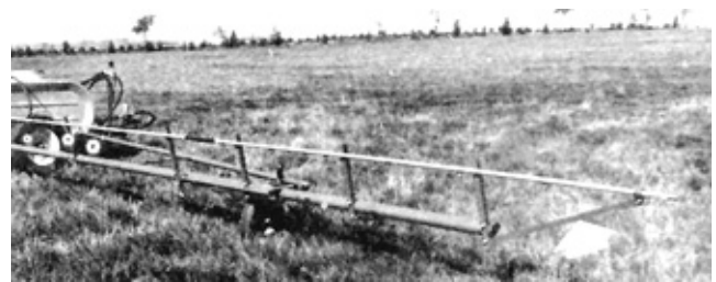
Figure 11. Boom End Braces.
