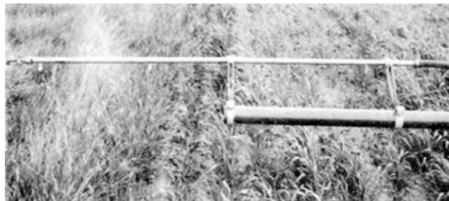
Figure 11. Unsupported Boom Ends.
