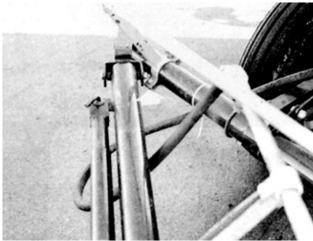
Figure 20. Short Turn in Transport causing Bending of the Boom Universal Joint.
