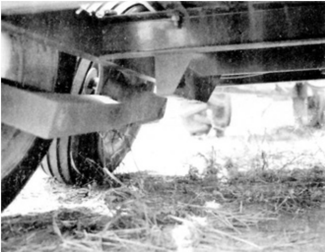
Figure 17. Damage to Rocker Axle.
