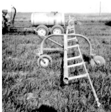
Figure 19. Bowed Boom Support Tube.
