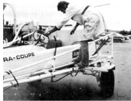
Figure 16. Awkward Mounting in Transport.
