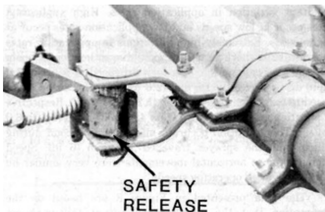
Figure 9. Safety Release on Radius Arm.
