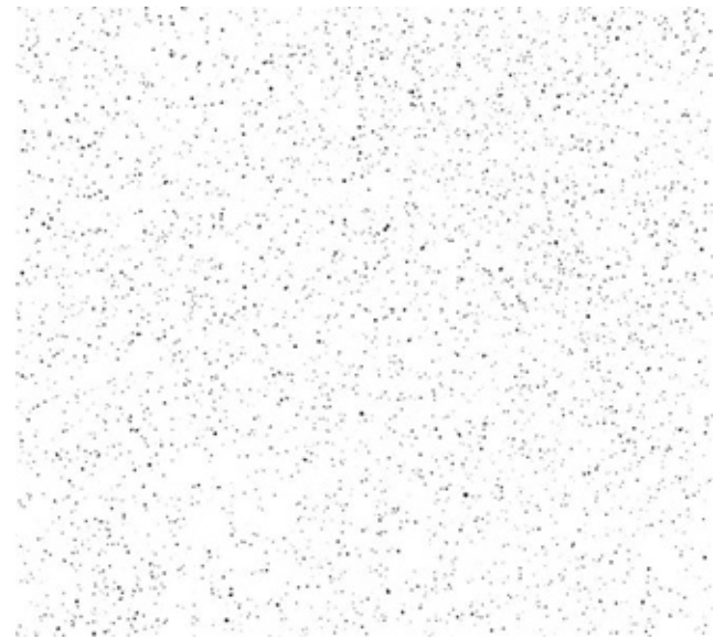
FIGURE 21. Droplet Sizes Produced by the Micromax when Spraying at the High Speed (7600 rpm) with the 4916-20 Orifice Plate.
