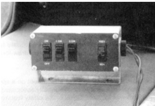
FIGURE 4. Remote Pump Control Box Mounted in Tractor Cab.
