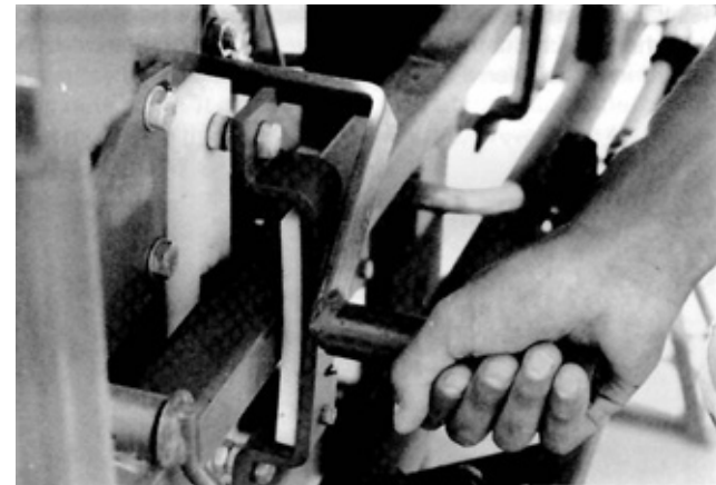
FIGURE 12. Winch Crank and Boom Frame Interference.
