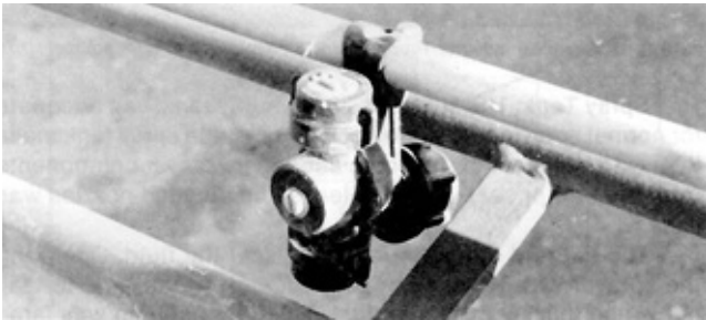
FIGURE 9. Application Rate Control System: (1) Pressure Gauge Green Zone, (2) Application Rate Decal, (3) Control Valve.
