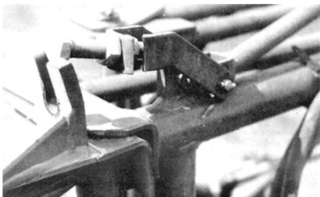
FIGURE 19. Failed Boom Lock Bracket.
