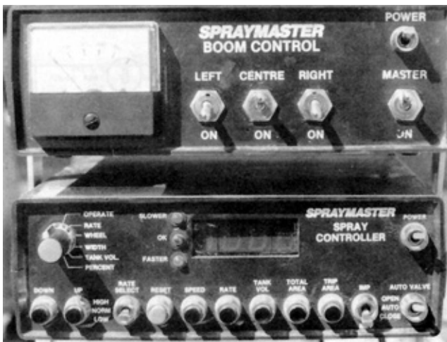
FIGURE 14. Computronics International Remote Control (upper) and Automatic Application Rate Controller Consoles (lower).
