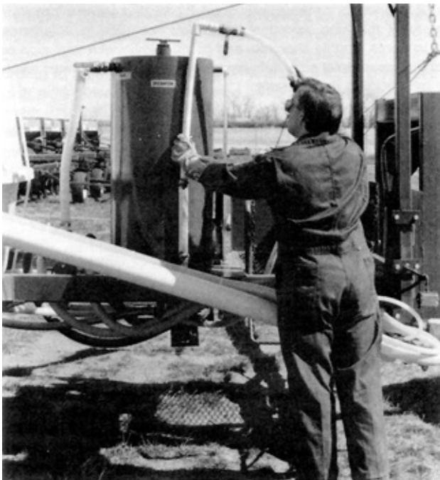
FIGURE 17. Operator Using Chemical Inductor Wand.
