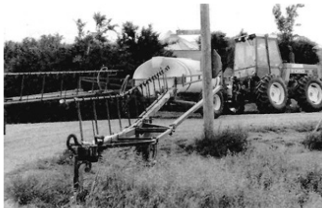
FIGURE 11. Inside Boom Position During A Sharp Turn.
