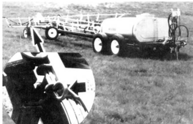
FIGURE 13. Wilger 804S Folded into Transport Position Showing Detail of Boom Wheel Lock Pin.
